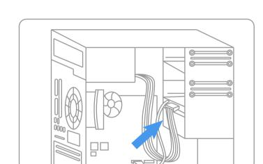
Step 3. SATA cables of the motherboard should be connected to the SATA data and power connectors on the solid state drive. Please be aware that the L-shaped SATA connector can only fit in one direction. Before pressing them into position, be sure to align the SATA plugs and solid state drive connectors properly.
