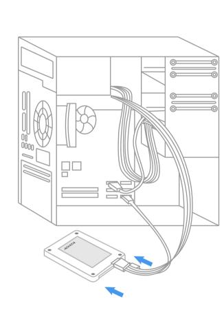
Step 4. The Solid State Drive can be securely mounted with the screws provided.
